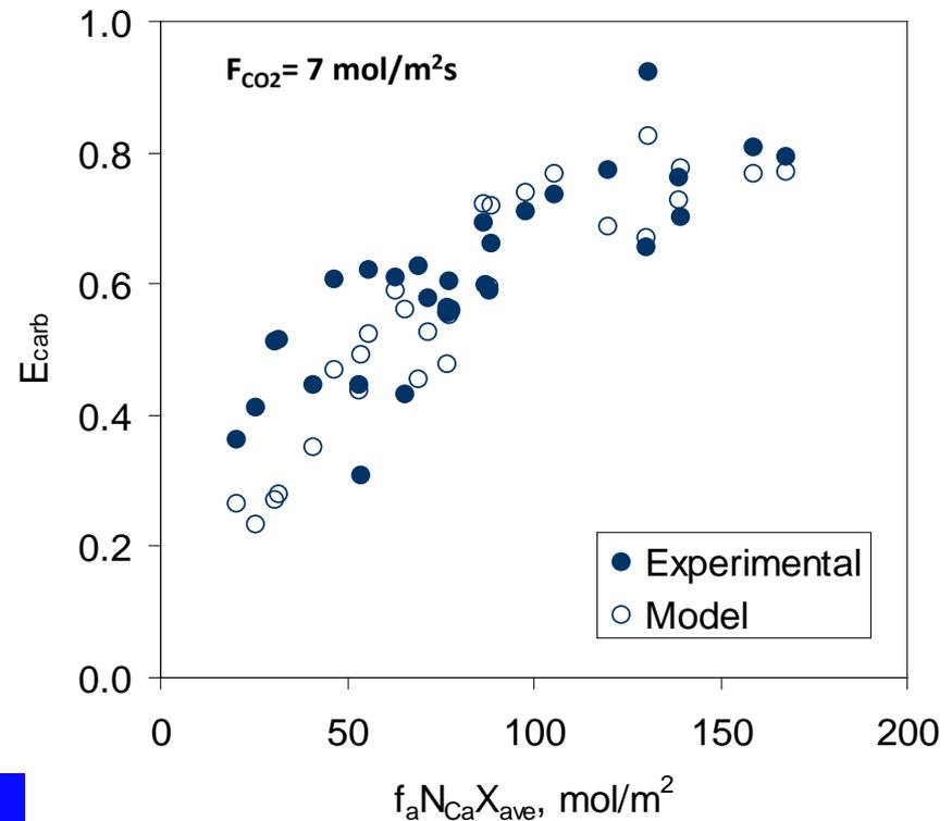
The CO<sub>2</sub> capture in the reactor is controlled mainly by the kinetics of the carbonation reaction
