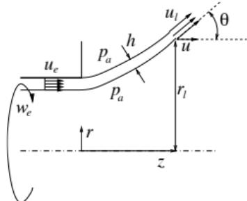
$$\mathcal{S} = \frac{w_e}{u_e} = \left( \frac{\Gamma r_i}{Q} \right)^{1/3} = \sqrt{\frac{r_i}{h_e}} \gtrsim 1$$
