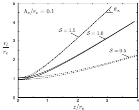
$$\frac{dr_l}{dz} = S \sqrt{1 - \left(\frac{r_i}{r_l}\right)^2}, \quad r_l(0) = r_i$$
